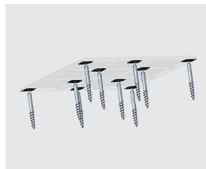
Juno screw foundation 2) The screw foundation contains the ground screws. Support brackets, fixing material and the screw-in aid
